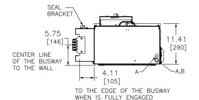
NOTES: FINISH — GRAY BAKED ENAMEL POWDER COAT PAINT OVER CLEANED GALVANNEALED STEEL. UL LISTED — FILE E131840, VOL. M MAIN HORIZONTAL CROSS BUS RATED AT 800 AMPERES. ALUMINUM  $1/4 \times 1-3/4$  TWO LAMINATIONS MAIN DEVICES ARE SEALABLE BY UTILITY.
