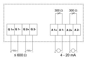
You can configure the following analog outputs on your meter through communication only:
