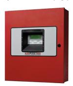
The fire panel controls the fire detection and extinguishing system. The panel can monitor two distinct areas, can trigger at least 2 levels of alarms, and incorporate a delay to evacuate the room before activating the extinguishing system. The system can also be activated by a manual switch attached to the panel.
