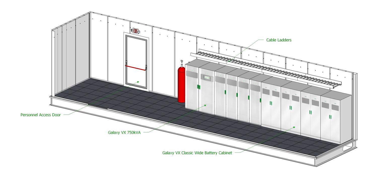
THIS DRAWING AND SPECIFICATION HEREIN ARE THE PROPERTY OF SCHNEIDER ELECTRIC AND SHALL NOT BE COPIED, REPRODUCED OR USED IN WHOLE OR IN PART AS THE WRITTEN PERMISSION FROM SCHNEIDER ELECTRIC. THIS DRAWING IS BASED UPON LATEST AVAILABLE INFOMATION AND REVENUE BASED UPON LATEST AVAILABLE BASED UPO
