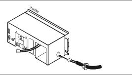
• Firmly push the two battery connectors together.
