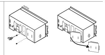
2 Remove the knockout panel that will be most convenient for connecting the external battery.
