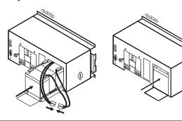
**4** Close the battery compartment door and secure the door with the two screws removed in step **1**.
