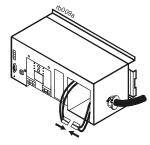
**6** Close the battery compartment door and secure the door with the two screws removed previously.
