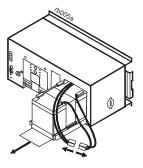
3 Slide the battery part way into the UPS. Be sure the battery connectors remain outside the UPS chassis. Firmly push the two battery connectors together. Slide the battery into the UPS.
