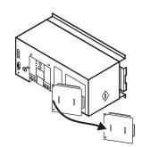
2 Pull the battery out of the compartment to access the battery connectors. Disconnect the battery.
