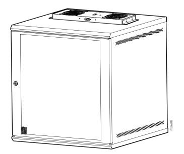
4. Secure the fan module to the top of the cabinet with the four (4) Phillips head screws. Torque to 3N•m.
