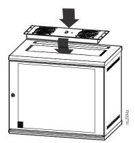
Secure the fan module with the Phillips head screws (provided). Torque 3N•m.
