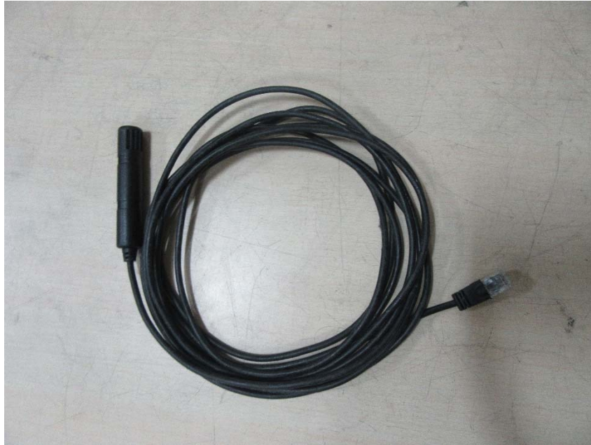
Figure 37: Photograph of Universal I/O port cable 1
