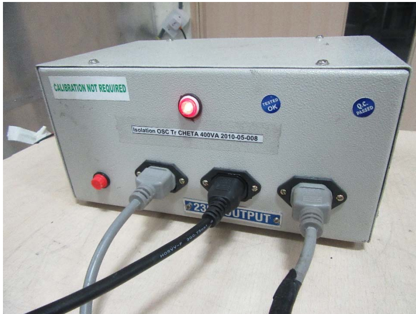
Figure 28: Photograph of isolation transformer
