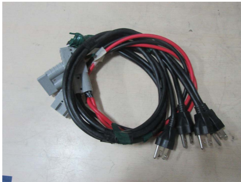
Figure 40: Photograph of AC output cable
