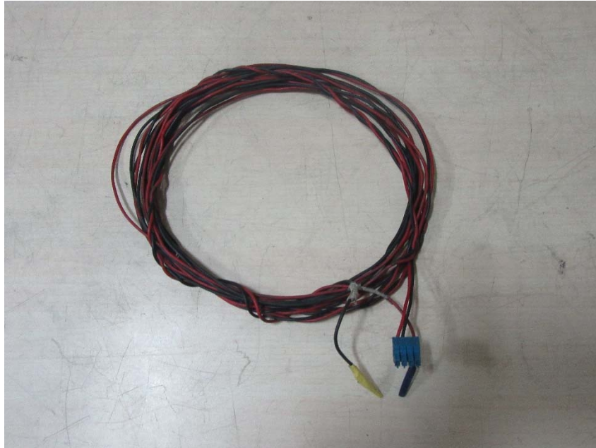
Figure 41: Photograph of EPO cable
