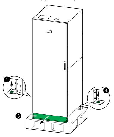
4. Remove the screws that attach the two rear anchoring brackets to the pallet.
