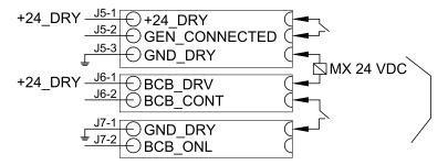
a. Connect the Aux switch signal cables from the empty classic battery cabinet to J6–2 and J7–1 in the UPS.
