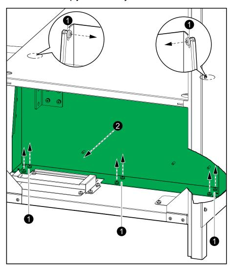
2. Remove the battery breaker plate.
