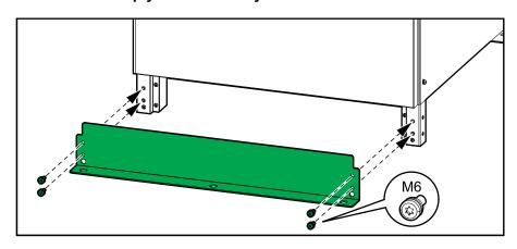
3. Anchor the front anchoring bracket to the floor.
