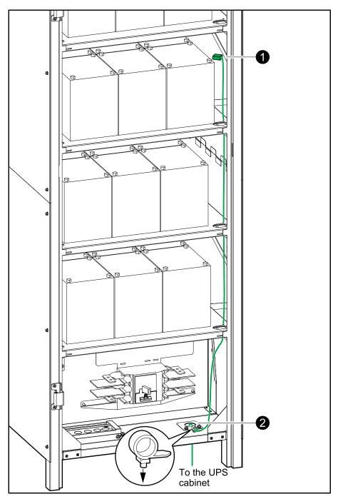
Route the battery temperature sensor cables through the top or the bottom of the empty classic battery cabinet to the UPS dry contact terminal J2–1 and J2–2 and connect as shown.
