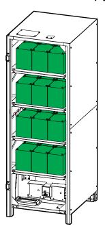
2. Connect the battery cables (Batt+, N, Batt-) from the batteries in the empty classic battery cabinet to the battery breaker.
