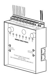
5. Connect a suitable ground or PE wire to the #8-32 ground stud in the lower left corner of the EPO box.
