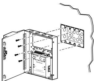
7. Reinforce the EPO box with 6 mm (¼ in) screws in the corner mounting holes.
