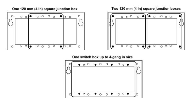
1. Install a junction box or a switch box behind the wall. The EPO box will fasten directly to the box. Use one of the options above. 2. Run the conduits (or cables) from the connected devices to the junction or switch box. If using conduits, it will contain all wiring from the connected devices and all cascading cables. Remove the knockouts required for installation.
