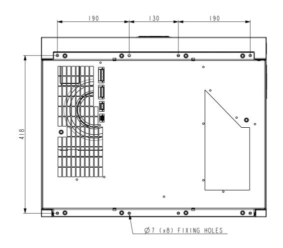
\* Requires to rivet 8x M6 blind popults in the enclosure roof at the position of the fixing holes.
