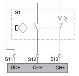
If the level at terminal S12 is logically 0 and the level at terminal S13 is logically 1, the safety-related input is activated.
