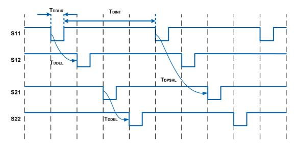
The diagram presents the input channels S11-S12 and S21-S22. The remaining input channels S13 and S23 as well as the remaining safety-related inputs S31-S32-S33, S41-S42-S43, S51-S52-S53, and S61-S62-S63 use the same logic as the input channels and safety-related inputs illustrated.
