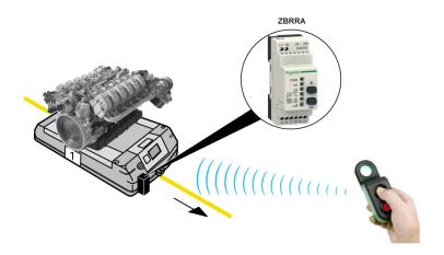
**NOTE:** When several AGV are in the same zone, use the 4 independent outputs of a ZBRRC receiver to correctly manage the AGV by the correct pushbutton.
