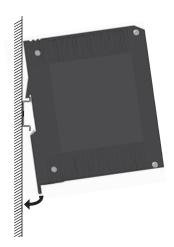
Figure 6: Mounting on the DIN rail
