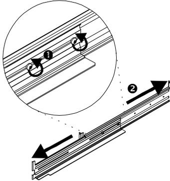
Remove the two screws ❶ that hold the rails together so that the rails can slide outward ❷. Do not detach the rails.
