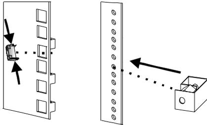
If your rack has round holes, insert clip nuts
