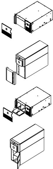
1. Remove the front bezel by grasping the finger clips on the side of the bezel and carefully loosening the four (4) snaps.
