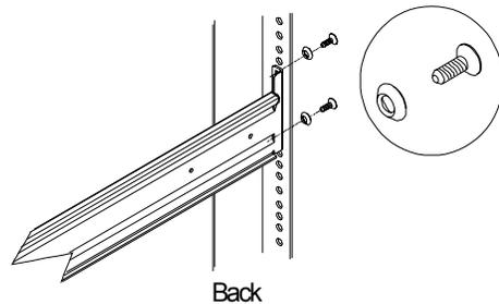
Attach the rail to the back rack post using the same hardware (10-32 flat head screws and conical washers) used in step 2. Repeat the process for the other rails.
