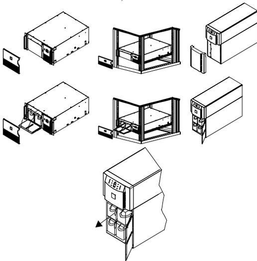
1. Remove the front bezel by grasping the finger clips on the side of the bezel and carefully loosening the four (4) snaps.
