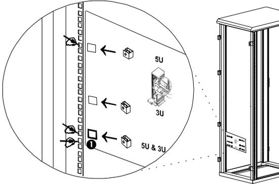
1. Determine where in the rack you'll mount the UPS. The SU5000 requires a space of 5U. Some racks have tick marks to indicate the U-spaces.
