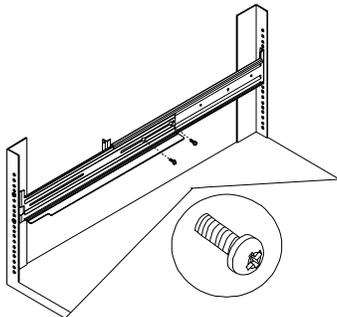
Expand the rails so that it spans from the front rack post to the back rack post. Replace the two screws (removed in step 1) that hold the rail sections together.
