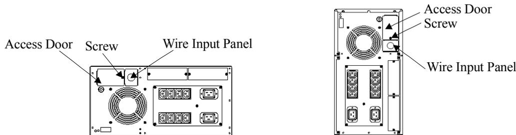
3. Slide the wire input plate to the left on rack mount units and up on towers and remove it. This will expose the input wiring terminal.
