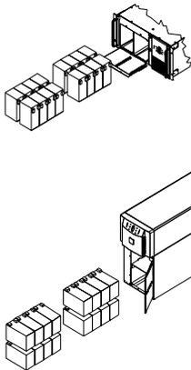
6. Replace the back battery pack. For rack mount units, hold a battery pack so its battery leads are on the right-hand side and slide it into the UPS. For tower units, hold the battery such that the battery leads are on the top and slide it into the UPS. Push the battery pack to the back of the compartment.
