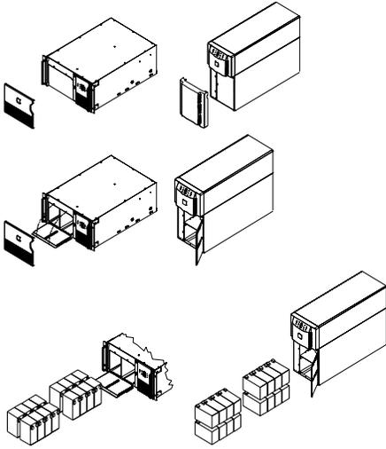
1. Remove the front bezel by grasping the finger clips on the side of the bezel and carefully loosening the four (4) snaps.
