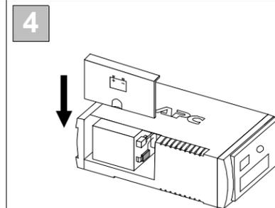
Align the battery compartment cover with the grooves in the UPS. Slide the cover down until it locks.
