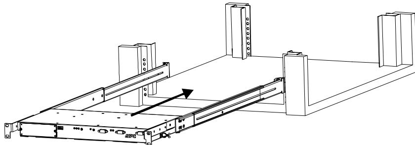
5. Secure the Redundant Switch into position by inserting two ornamental (10-32) screws through the front of the mounting bracket on each side.
