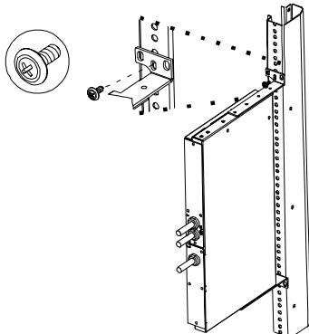
1. Place the Redundant Switch vertically on the rear rack post. Position the front of the Redundant Switch against the rack post so that the rear panel is accessible.
