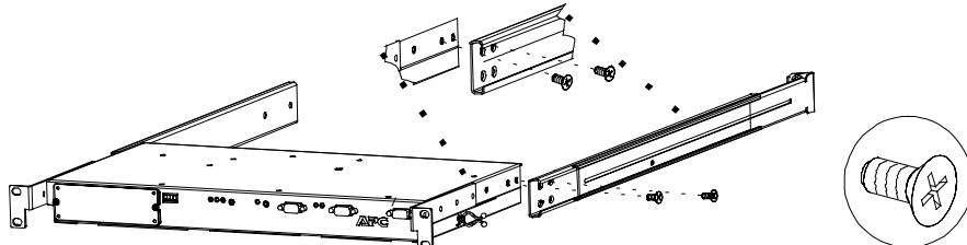
4. Support the Redundant Switch from the bottom or rear of the unit and slide it into the rack.
