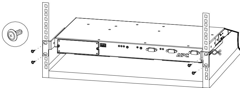
6. From the rear of the rack, extend the rear rail segment to the rear rack post. Use the (flat head screws #10 x 1/2") and cup washers provided, to attach the rail to the rack post.
