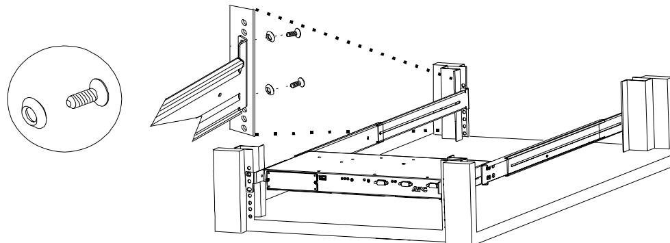
7. Insert and tighten the slide screws and nuts to secure the front and rear rail segments.
