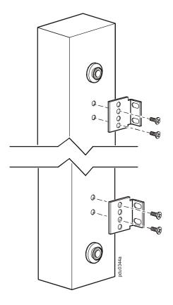
Install the Rack PDU on a vertical mounting rail in your rack or enclosure using the supplied screws and caged nuts.
