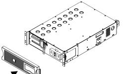
4. The UPS is shipped with the front bezel removed (it is packaged separately within the main box). Unpack the bezel and hold it with the cutout section on the right. Align the tabs on the side of the bezel with the slots on the front of the UPS and gently snap it into place.
