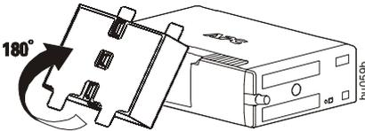
3 Flip or turn the battery 180 degrees upward/downward to let green side of the label face up.
