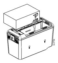
3 Reinstall the battery compartment cover. Be sure that the release tabs lock into place.
