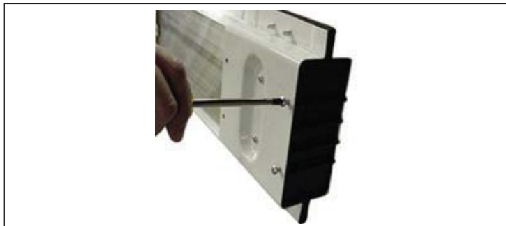
Figure 14: Tightening the Plastite® Thread-Rolling End Screws
