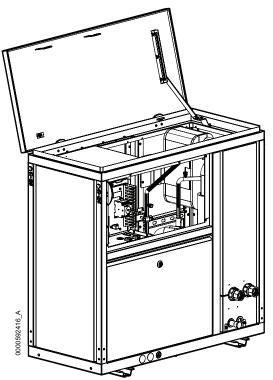
5. Remove the electrical box top panel.
