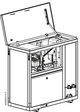
5. Remove the electrical box top panel.
