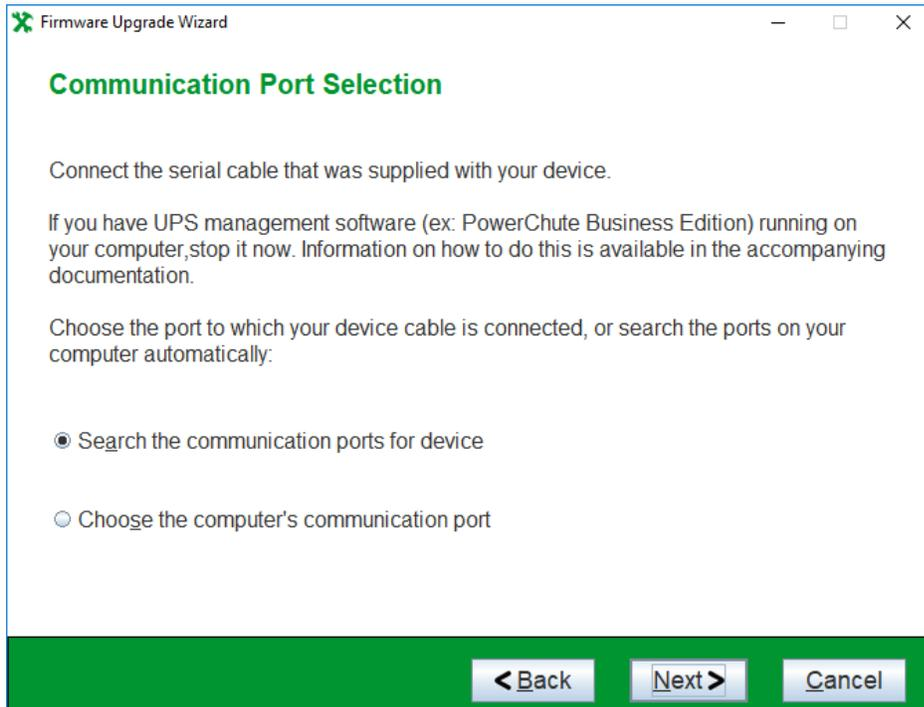
The Firmware Upgrade Wizard will now search the communication ports for the UPS. The UPS is referred to on-screen as the “device”. If you have set up virtual ports, it is important to manually select the correct port, the UPS is connected to, here.
