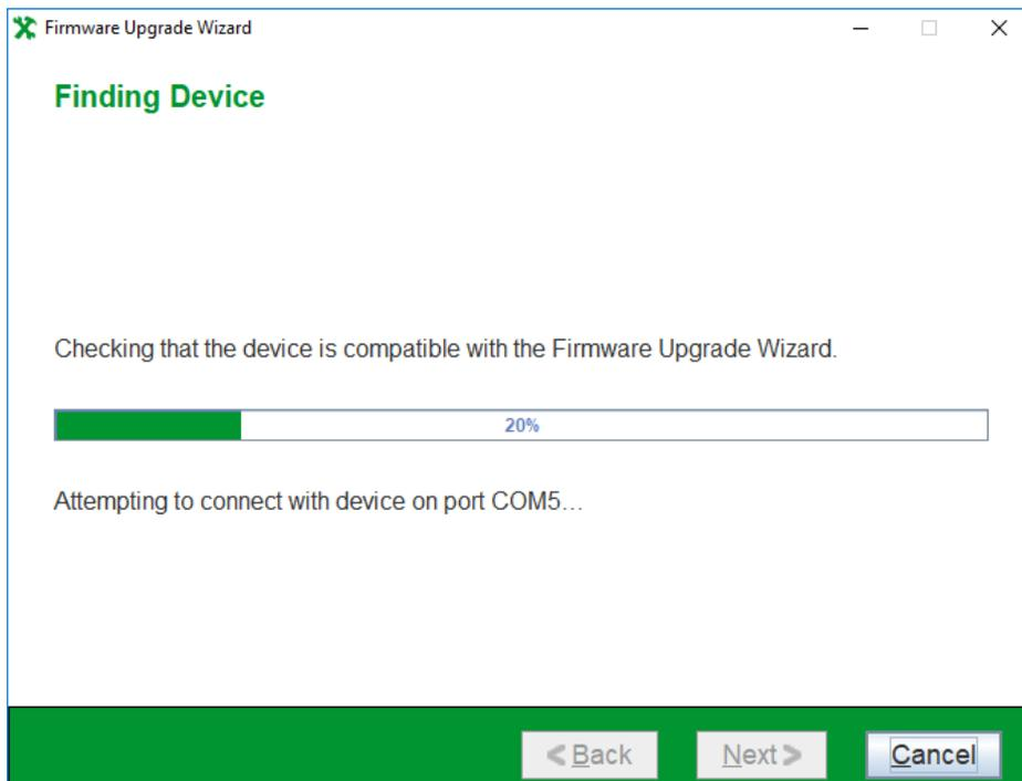
Click “Next” and the Firmware Upgrade Wizard will display the current firmware version installed on the device.
