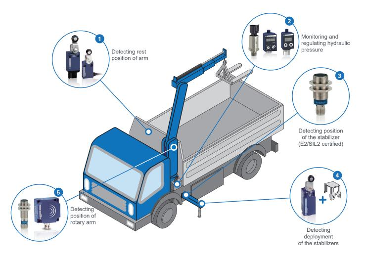
XCMV or XCMD Limit Switch Compact body and modular head allows easy mechanical adaptation.
