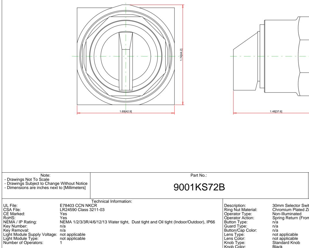
Specification: Description: Ring Nut Material: Operator Type: Operator Action: Button Type: Guard Type: Button/Cap Color: Lens Type: Lens Color: Knob Type: Knob Color: 30mm Selector Switch Chromium Plated Zinc Non-Illuminated Spring Return (From Right to Center) NEMA 1/2/3/3R/4/6/12/13 Water tight, Dust tight and Oil tight (Indoor/Outdoor), IP66 n/a n/a n/a not applicable not applicable Standard Knob Knob Color: Black Number of Positions: 3
