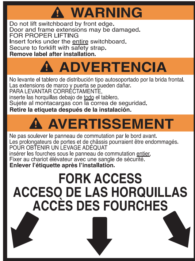
Figure 4: Warning Instruction Label, Rainproof Switchboards
