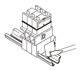
To install end clamp, insert U-shaped portion of clamp between mounting track and terminal block. With screw driver inserted in slot as shown, apply force toward track and block, sliding end clamp tight against side of terminal block.
