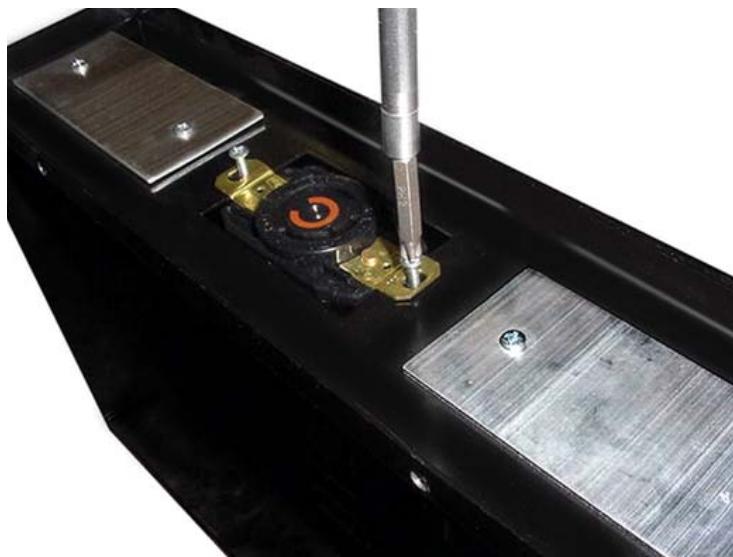
Figure 42: Plug-in Unit Receptacle Installation Location
