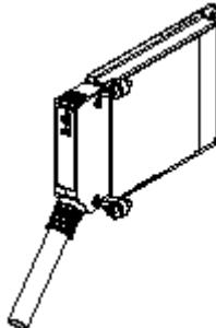
**Warning:** The PCMCIA board must be manipulated only when the XBT is powered off.
