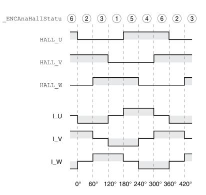
The encoders of third-party motors may deliver a different pattern even though the designations *HALL\_U*, *HALL\_V* and *HALL\_W* are used. In such a case, the encoder pins *HALL\_U*, *HALL\_V* and *HALL\_W* must be wired differently.
