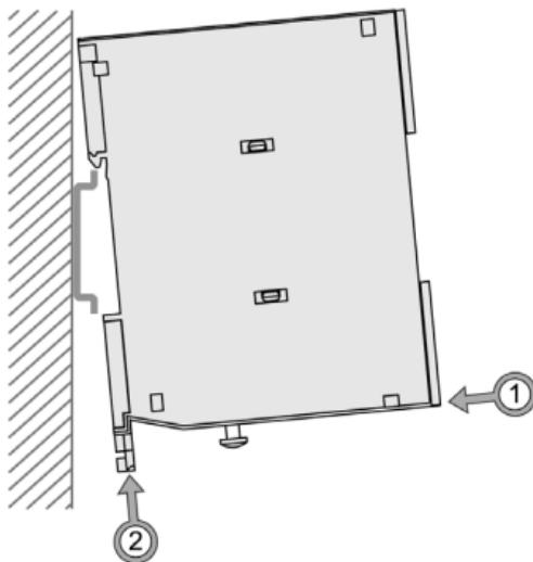
Usually, TwidoPort is mounted on a DIN rail or a panel with the Twido panel mount kit (TWDXMT5).
