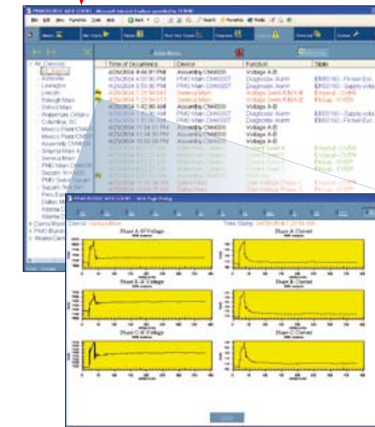
Alarms show active status and alarm history. The alarm log includes waveform analysis links to aid troubleshooting power quality system events.
