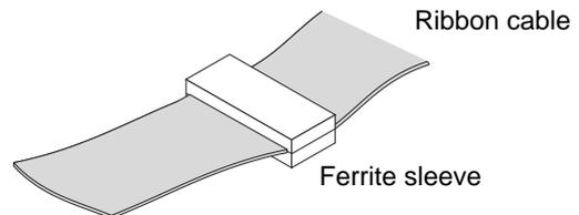
Half-shell ferrite sleeves are easier to install but less effective than solid (enclosed) ferrite sleeves.
