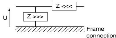
Equivalent high-frequency (HF) circuit diagram
