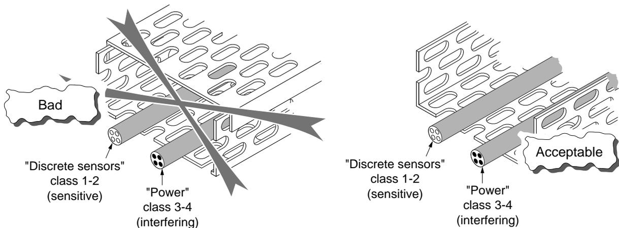
If «sensitive» (class 1-2) and interfering (class 3-4) cables are laid in the same cable trough despite the fact that this is not at all recommended, it is then preferable to leave the cable trough open.
