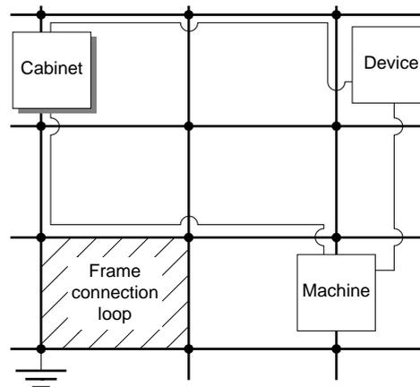
***Loops between exposed conductive parts are the result of systematic, careful interconnection to ensure equipotential bonding at a site***
