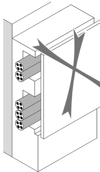
Moulding, skirting (jamb lining) with grooves
