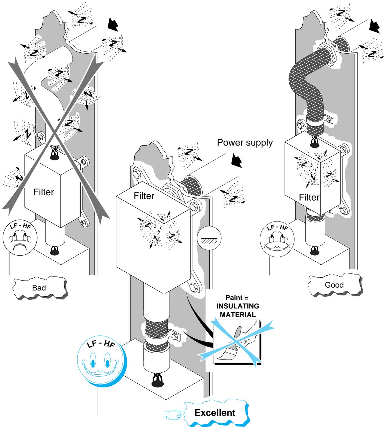
Filters must be fitted at the point where cable enters the cabinet and be bolted to the chassis or earth plane at the bottom of the cabinet
