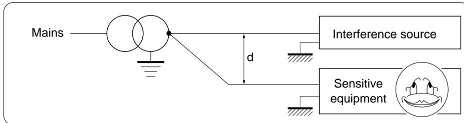
$d$  = distance between cable: [see Wiring rules later on in this chapter.](#)
