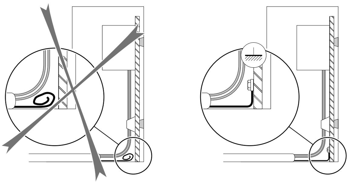
For class\* 1 signals, such connection may generate LF buzzing superimposed on the useful signal if the equipotential bonding of the exposed conductive parts of the installation is inadequate.
