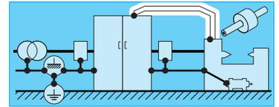
Interfering and sensitive cables must be laid along separate cable routes.
