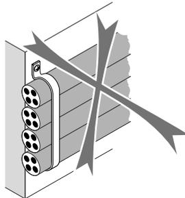
Direct attachment to walls and ceilings using clips, ties, etc.
