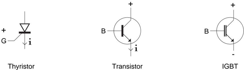
IGBT = Insulated **G**ate **B**ipolar **T**ransistor
