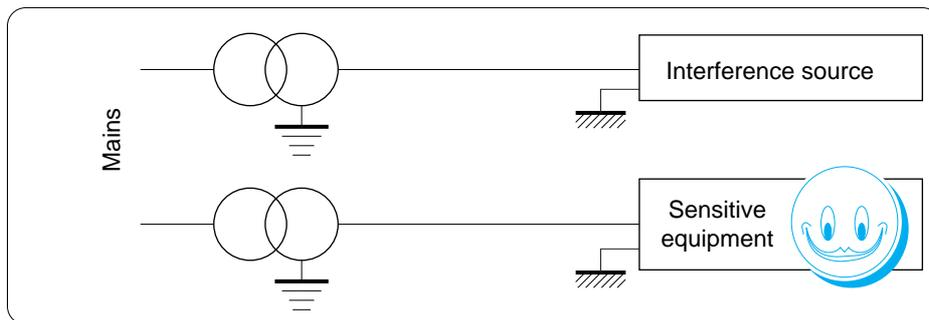
Wire the supply circuits by placing interfering equipment as close as possible to the power source and the most sensitive equipment farthest from the power source.
