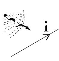
Conductor = "receiving" antenna
