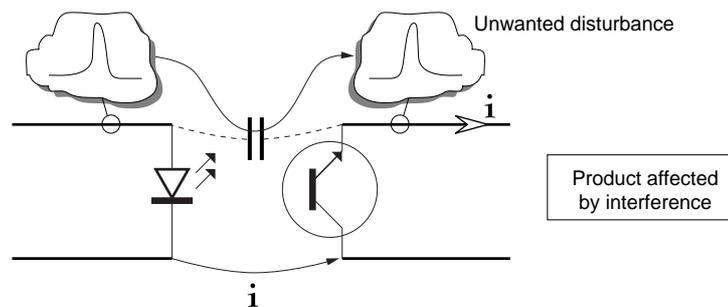
The phenomenon is the same with optocouplers although their low-frequency (LF) impedance and high-frequency (HF) performance are generally better than those of signal transformers.
