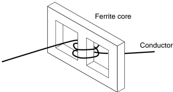
The number of turns increases the effectiveness but also creates stray capacitance between turns. The max. number of turns not to be exceeded depends on the :
