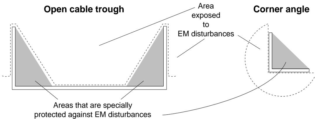
The shielding, protective or screening effect of a metal cable trough depends on the position of the cable.
