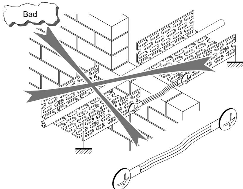
A conductor that is roughly 10 cm long reduces the effectiveness of a cable trough by a factor of 10.
