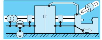
**4** Maximise the distance between cables carrying signals of different classes\*, especially sensitive signals (1-2) and interfering signals (3-4) - this is very effective and relatively inexpensive.
