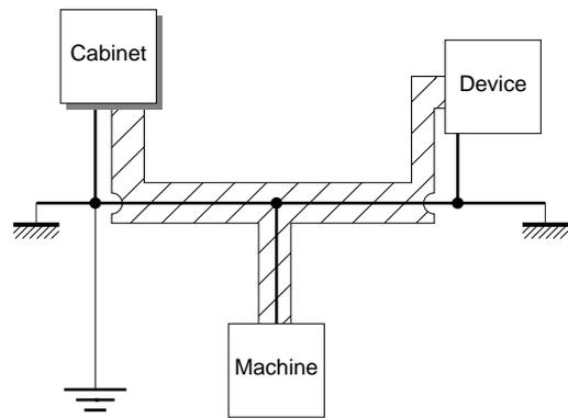
Place all conductors against the earth plane end to end (panel at bottom of cabinet, exposed conductive parts of metal enclosures, equipotential structures of machine or building, accompanying conductors, cable troughs, etc.).
