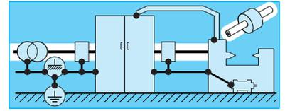
**6** The *OUTGOING* conductor must always be routed as close as possible to the *RETURN* conductor.
