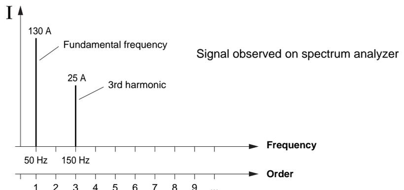
*Harmonic interference is low-frequency (LF) type interference and is therefore mainly «conducted».*
