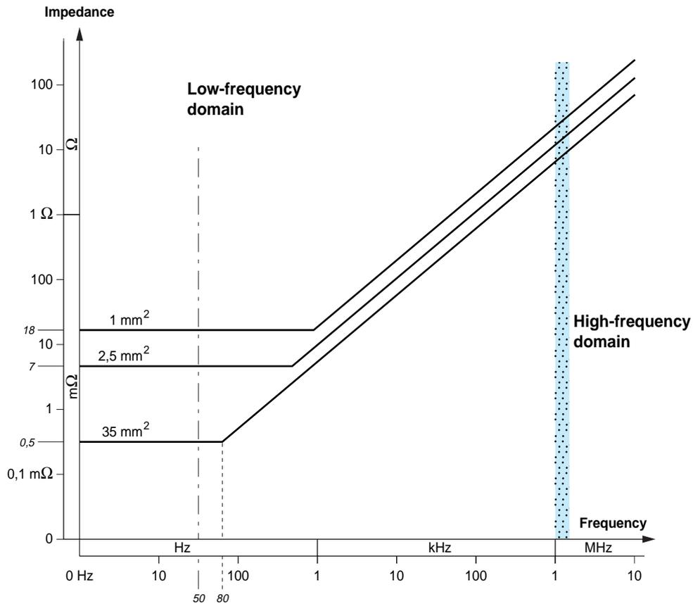
Typical impedance values of an electrical conductor of length  $L = 1 \text{ m}$
