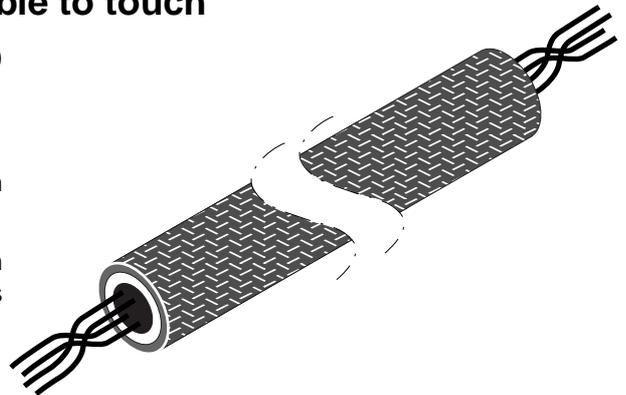
*Completely ineffective, especially when compared with capabilities of correctly fitted shielding and its cost.*
