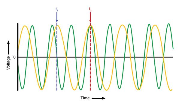
Figure 1: In-rush current at  $t_1$ , where the phase angle difference is~90 degrees, would be much greater than at  $t_2$ , where the difference approaches zero degrees. In normal applications, the frequencies would vary less widely than shown.
