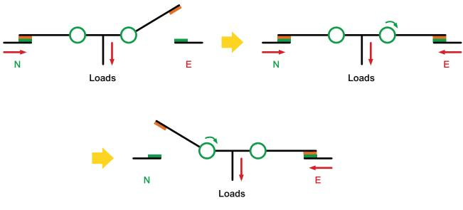
Figure 4: A closed transition sequence where the Normal and Emergency sources are momentarily paralleled.
