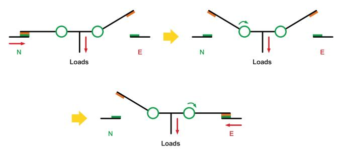
Figure 3: A delayed transition sequence, where the transfer mechanism contacts disconnect from the Normal source, hold a center-off position, then connect to the Emergency source.
