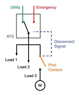
Figure 2: A motor load disconnect circuit solution
