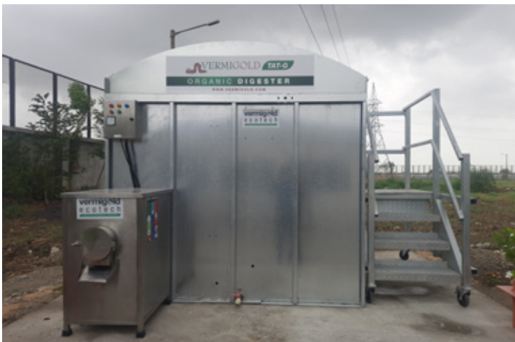
➤ Vermicomposting plant in MVI site
