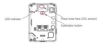
Start flowing nitrogen gas (0 ppm CO<sub>2</sub>). Use a flow rate of 0.3 to 0.5 liters/minute.
