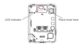
\*Note that the CO<sub>2</sub> sensor has an optical bench that flashes. This is not the LED. The LED is at position D6 on the board. See diagram above.
