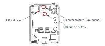
Start flowing nitrogen gas (0 ppm CO<sub>2</sub>). Use a flow rate of 0.3 to 0.5 liters/minute.
