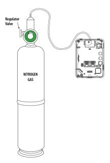
Press and hold down the calibration button. The LED\* will turn off. Hold for five seconds. After holding down the calibration button for two seconds the LED will flash once. Continue to hold. After holding down the calibration button for 5 seconds the LED will flash twice. Release button and the 0 ppm calibration process begins. The LED flashes slowly to indicate calibration is in progress.
