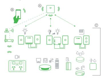
The Wiser hub (see A) is the center of the system, processing control requests and status reports for connected Wiser devices.
