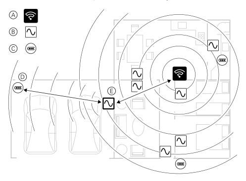
**TIP:** The battery-powered motion sensor in the garage (D) is a long way from the hub. However, the sensor can connect to the hub via the mains-powered device being used as the garage light switch (E). This is because mains-powered devices also act as system network extenders. Consider this when deciding where to locate the hub.
