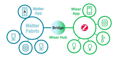
In this case, Wiser Hub 2<sup>nd</sup> Generation / Wiser Hub<sup>R</sup> 2<sup>nd</sup> Generation acts as the Matter Bridge. By adding the hub to a third-party Matter app (Google/Amazon/Apple etc.), you can integrate your Wiser Zigbee devices into the Matter Fabric (network) and control them from the third-party app.
