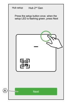
4. Connect your smartphone to the Hub's temporary Wi-Fi® network either by QR Code connection or Manual connection.
