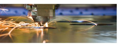
Cut-outs are created with digitally-controlled laser or punching machines. This helps ensure that the position and dimensions of cut-outs are accurate and strictly identical across all the enclosures with the same configuration. The cut-out edges don't require any touch-ups.
