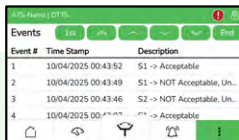
ATS Statistics with Event Log: Displays detailed information for 1000 events, including time of occurrence, duration, date, and reason.
