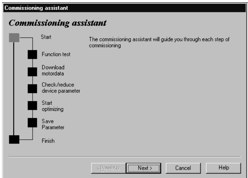
Fig. 5.5 Commissioning with the assistant in the Twin Line Commissioning Tool
