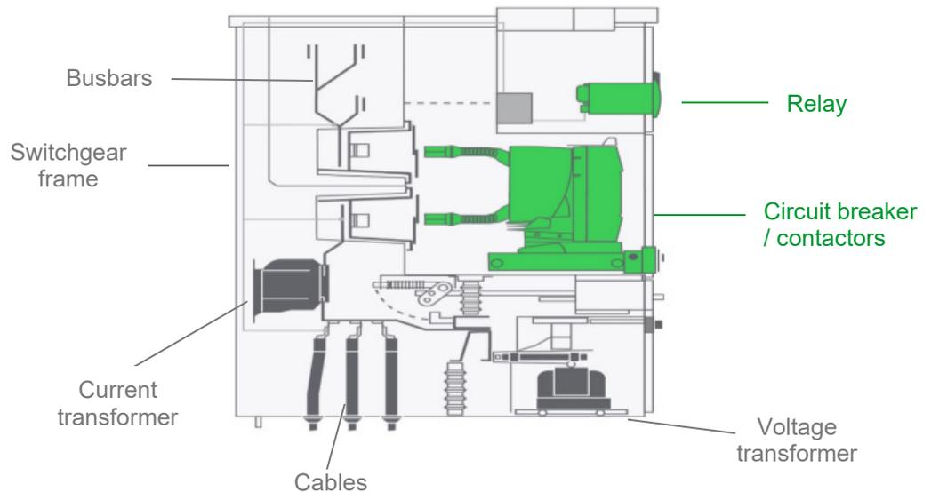
Rather than replacing the entire switchgear system, when these critical components approach their end-of-life, they can be either “retrofit” or “retrofitted”<sup>7</sup>, which has a lower environmental impact.
