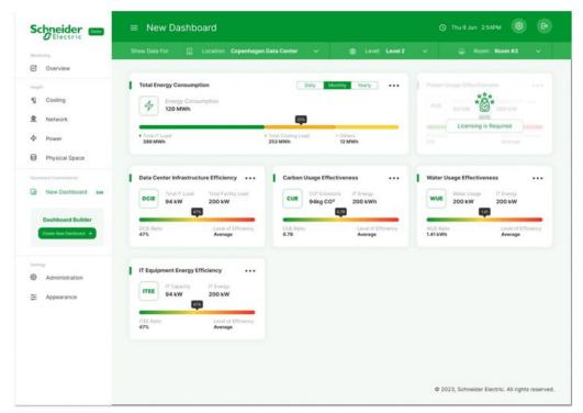
For these metrics to be meaningful, of course, it is important that the DCIM software be able to communicate with and normalize data from all power and cooling infrastructure devices, regardless of make or model. This ensures a complete picture of environmental impact. So DCIM tools and infrastructure devices that embrace common, open protocols (e.g., SNMPv3) and that accommodate the use of APIs/web services should be used.
