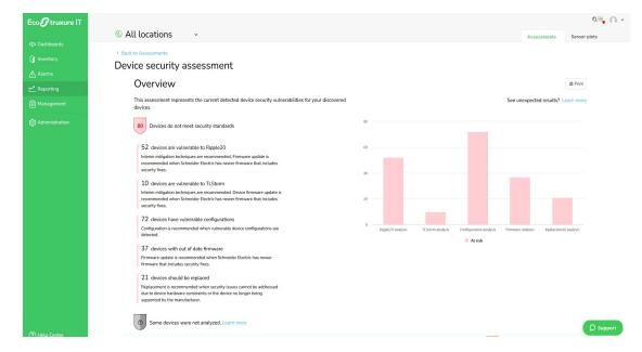
Some DCIM tools will also automate the updating of firmware and provide a means to perform mass configurations of security settings across multiple devices at once to greatly simplify the process. The more DCIM can simplify and automate these security processes, the more secure the physical infrastructure systems will be as it reduces the opportunity for human error.
