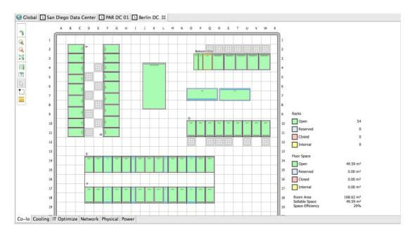
This overlay map of the IT space shows a breakdown by tenant, what space is reserved for future tenants, what is available to sell to new tenants now (as well as showing power/cooling capacity, network ports for a given zone, etc.) This gives the provider improved visibility to data center assets and capacity in real time yielding sales enablement and change management efficiency benefits.
