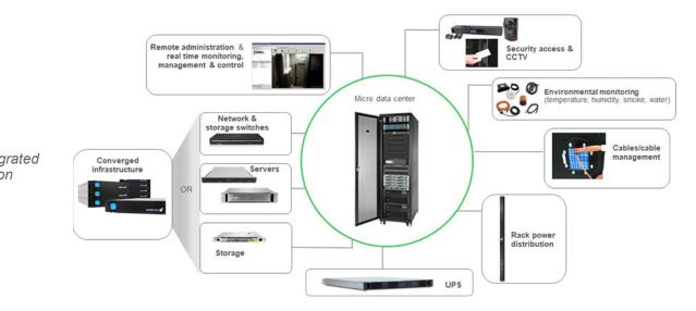
**Figure 8** Example of a fully integrated edge computing solution
