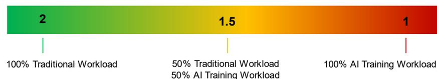
**GUIDANCE:** In the case of a new data center hall with greater than 60-70% of AI training workloads, we recommend sizing the main breaker based on the sum of the individual feeder breakers downstream. In other words, assume a peak-to-average
