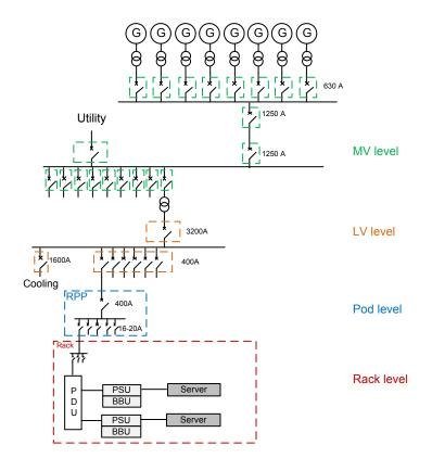
This architecture is not likely to be widely adopted, however, as it requires downtime of critical loads in order to conduct maintenance on many of the components in the upstream power path.
