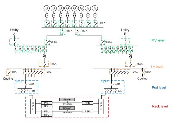
Note that although this design offers 2N power paths to the critical load, there is only 1N BBU. Removing the redundant BBU reduces capital expense.
