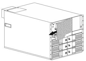
Loosen the thumbscrew to disable the module and unlock the latch.
