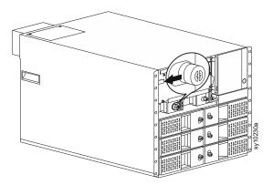
Release the latch and pull the finger hold on the front face of the module until the latch clears the frame.
