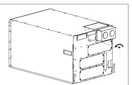
2 Remove the UPS battery connector cover.
