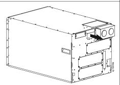
Insert the XBP power cable connector into the UPS battery connector.
