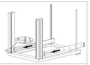
Secure the XBP rail to the rack with 12 flat head screws and conical washers (supplied).
