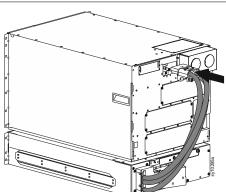
Tighten the thumbscrew to secure the XBP power cable connector to the UPS battery connector.
