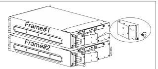
Remove the XBP battery connector cover in Frame#1.
