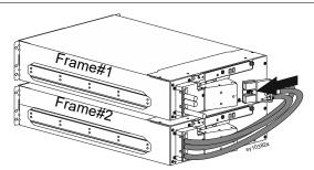
Tighten the thumbscrew to secure the XBP power cable connector of Frame#2 to the XBP battery connector in Frame#1.
