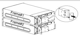
Insert the XBP power cable connector of Frame#2 into the XBP battery connector in Frame#1.
