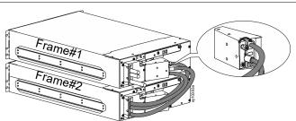
Set a unique identification (ID) number on the FRAME# SETTING switch (refer to "Rear Panel Features of XBP" section in the UPS user manual for location of this switch).
