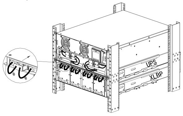
**5** Secure the battery compartment door with 9 screws.
