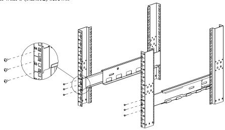
3 Secure the brackets on battery pack with 4 (M4x6) screws.
