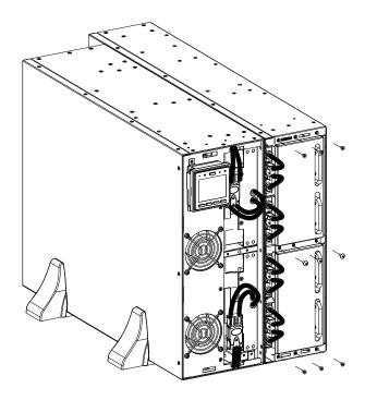
Install battery pack front bezel and UPS front bezel.
