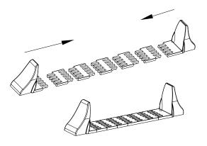
2 Mount the UPS and battery pack to the stabilizer bracket.
