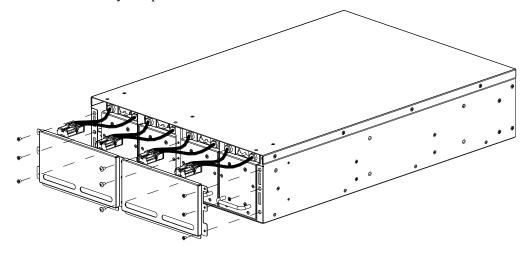
4 Remove the battery modules from the battery pack.
