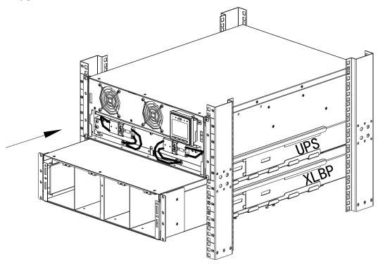
2 Secure brackets to pillar with 4 (M5x12) screws.
