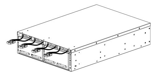
**3** Remove the screws and battery compartment door.
