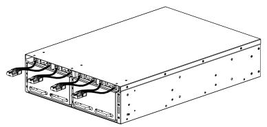
2 Remove the screws and the battery compartment door.
