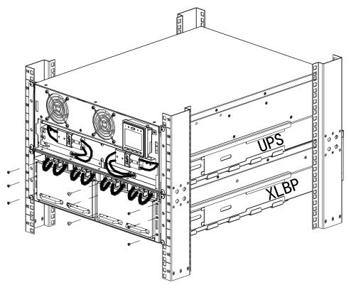
**6** Install battery pack front bezel and UPS front bezel.
