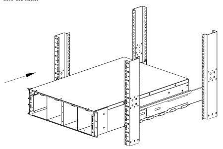
**5** Secure brackets to pillar with 4 (M5x12) screws.
