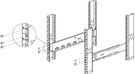
2 Secure the back of rail with 6 (M5x12) screws.
