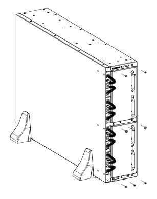
9 Install the front bezel of battery pack.
